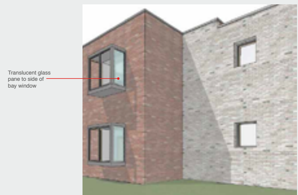
Illustration showing the translucent glazing side to the bay window at the end of the wing
